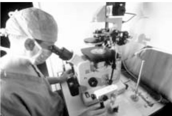
Figure 2. Embryo biopsies are performed by an Embryologist working with micromanipulators on an inverted microscope.
